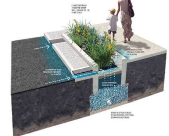
Typical Bioretention and Tree Well (Source: Philadelphia Green Streets Design Manual)
