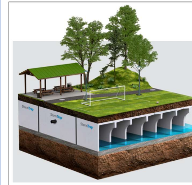
Typical Infiltration Gallery (Source: StormTrap)
