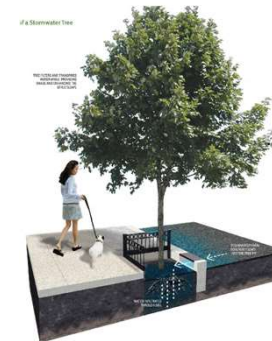
Typical Bioretention and Tree Well (Source: Philadelphia Green Streets Design Manual)
